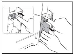
Press the lock button and gently remove the waste toner box.
